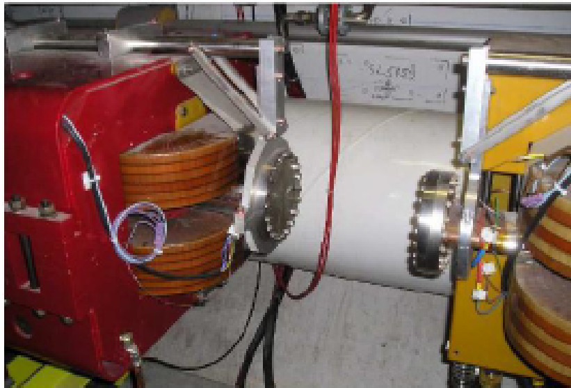
Accessible warm beam pipe between BMX magnets
