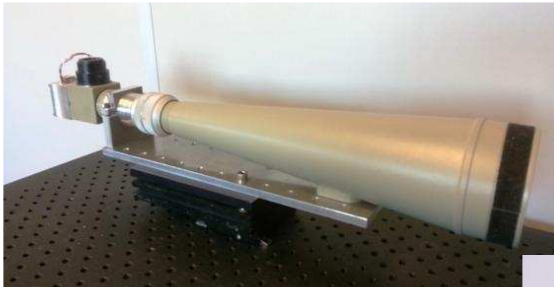
Optical autocollimator with improved sensitivity
