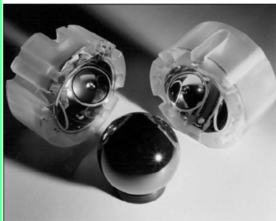
Gravity Probe B gyroscope (rotor), with quartz housing halves.
