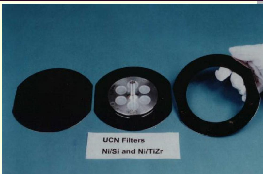
**Multilayer structures on a Si wafer.
