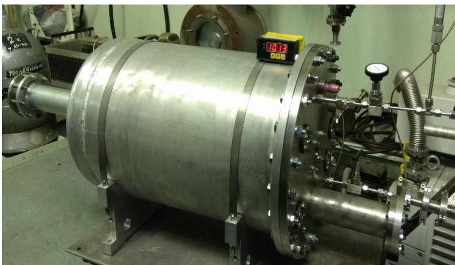
Fig.8. ACTAF2 in the test laboratory. The pressure inside ACTAF2 is 10.13 bar of argon. The side view of the ACTAF2 with the digital display and manometer for the pressure test.
