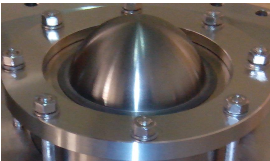
Fig.9. The picture of the Be window mounted on a flange of the pressure vessel.
