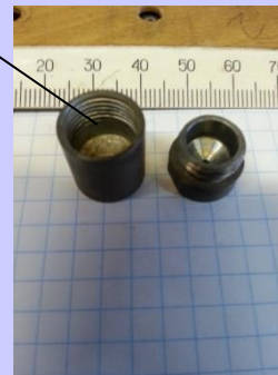
Cavity after heating at a temperature higher 900° C. Target material was completely evaporated
