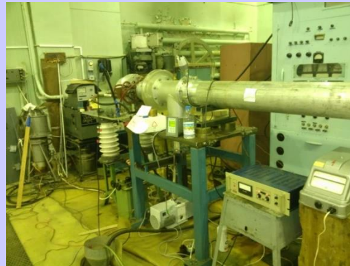
The first tests of accelerating voltage 30 kV with the target-ion source heating
