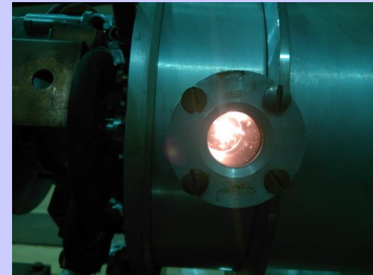
The first tests of accelerating voltage 30 kV with the target-ion source heating
