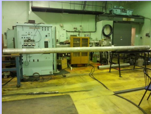
The first prototype of internal vacuum tube in the IRIS experimental hall
