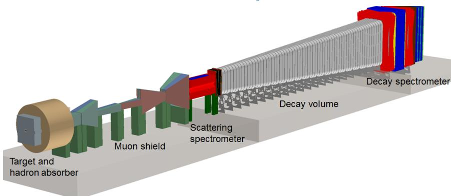
SHiP remains a unique dedicated experiment capable of reconstructing the decays vertex of hidden particle, measuring its invariant mass and providing PID of the decay products in zero background environment
