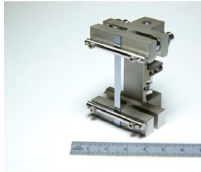
Strip crystal for the LHC (developed by INFN).
