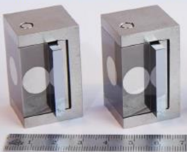
Crystal collimator prototypes developed by Russian Institutes for LHC
