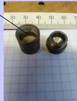
Cavity after heating at a temperature higher 900° C. Target material was completely evaporated
