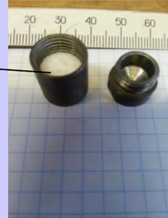
Cavity with RbCl before heating at a temperature lower 800° C
