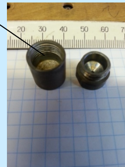
Cavity after heating at a temperature higher 900^\circ\text{C} . Target material was completely evaporated
