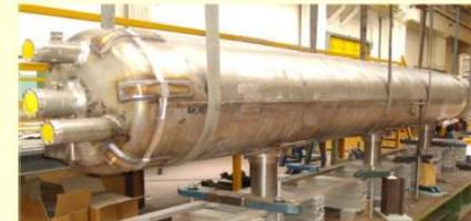
Full length curved, fast ramped s.c. SIS300 dipole magnet Delivery, July 2013
