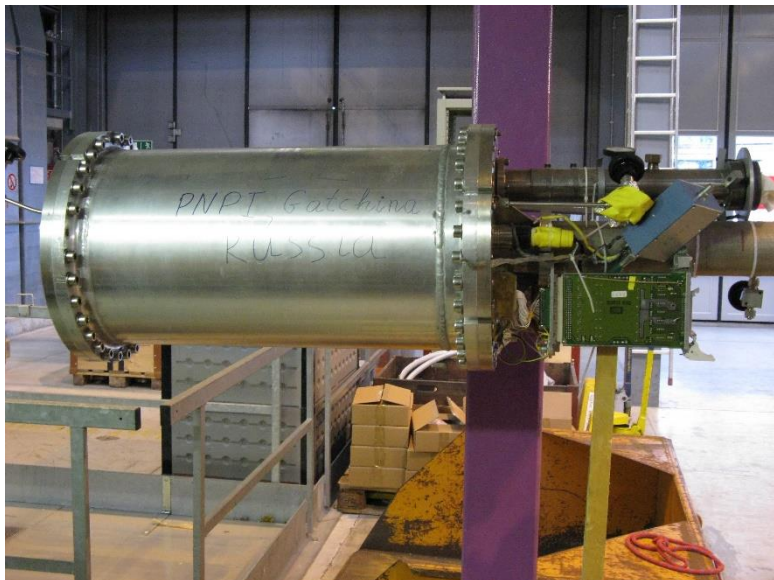
Прототип камеры ACTAR2 E_{\alpha} = 1-10 МэВ The length – 60 cm, the inner diameter – 28 cm, the working pressure – 10 bar.
