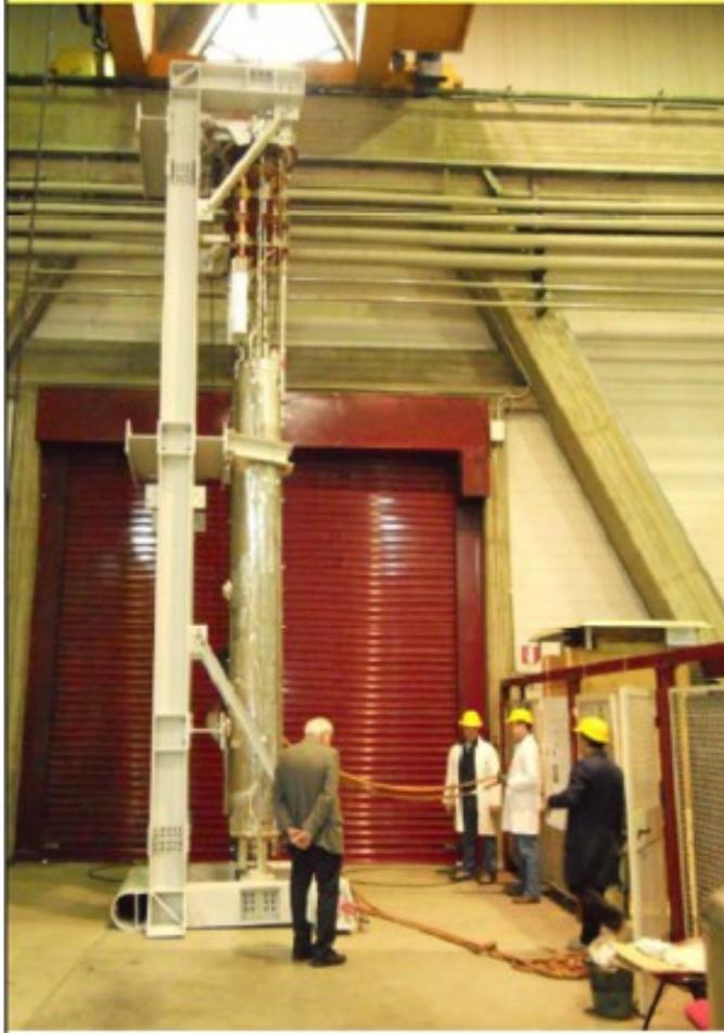
Preparation of a SIS300 quadrupole magnet
