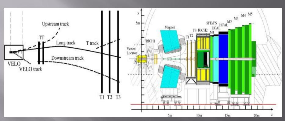
M1, M2, M3, M4, M5 – muon stations RICH1, RICH2 – Cherenkov detectors TT, T1,T2,T3 – tracking stations VELO (Vertex Locator) – vertex detector •The total integrated luminosity recorded -  $\int Ldt = 34 \ pb^{-1}$ .  $\int Ldt = 31 \ pb^{-1}$  used for the analysis
