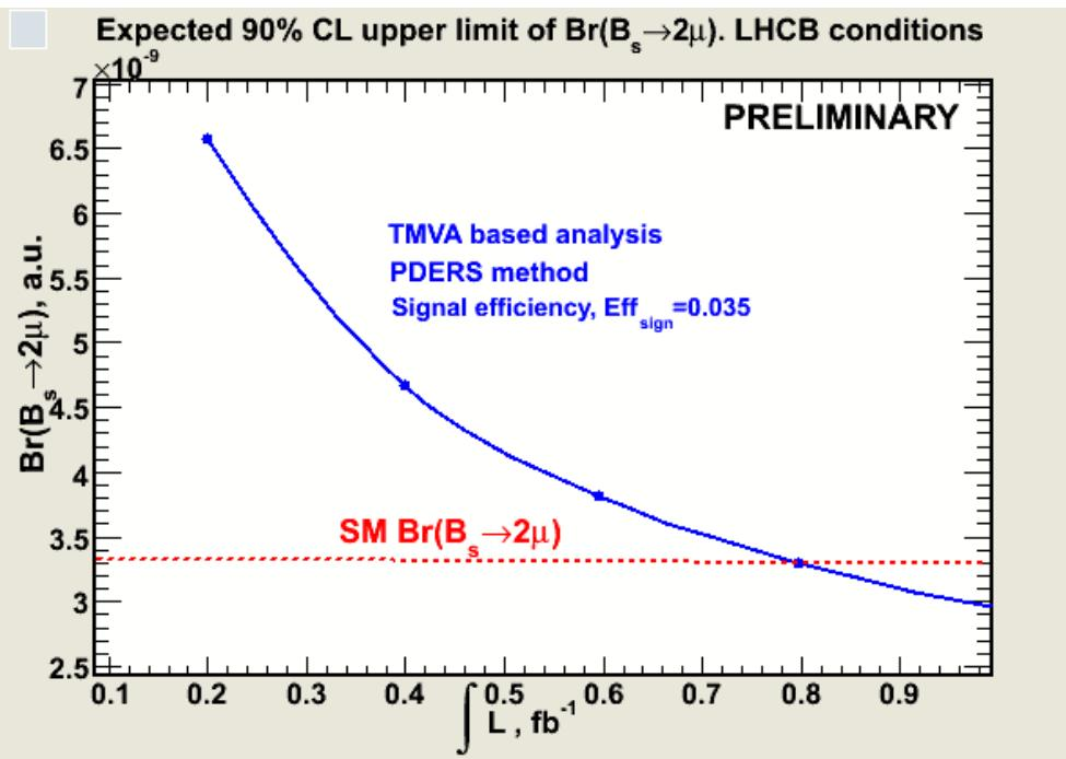
The predictions for the 90% CL upper limit for  $B_s \rightarrow 2\mu$  decay. We can reach the level of the SM branching at 1  $\text{fb}^{-1}$  (*PNPI group result*)
