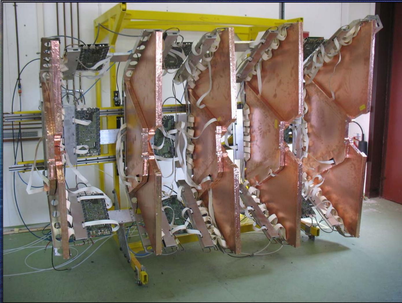
**ЦЕРН. Cathode strip readout electronics for
