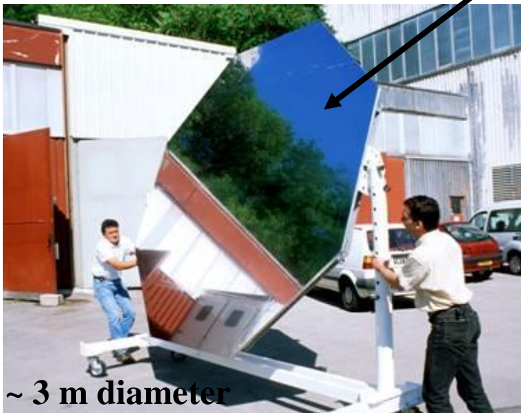
Central Electrode Prototype 25 \mu\text{m} aluminized Mylar on Al frame
