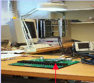
ALCT 384 on the Test Station
