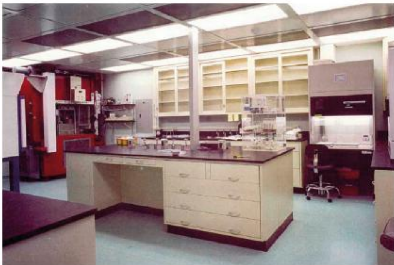
FIG. 1.10. A typical radiochemistry laboratory just after completion. (Note that the laminar flow hood on the right for the preparation of sterile vials and the red hot cell on the left where the syntheses are carried out.)
