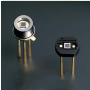
SiPM (HAMAMATSU U50) (400 pixels) Operating voltage ~70V
