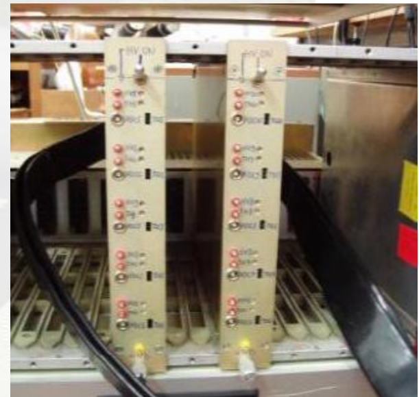
5 Channels HV power supply (stability better than 10 mV)
