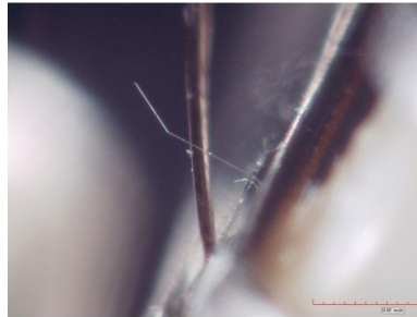
Optical comparison of Human Hair vs. Tin Whisker
