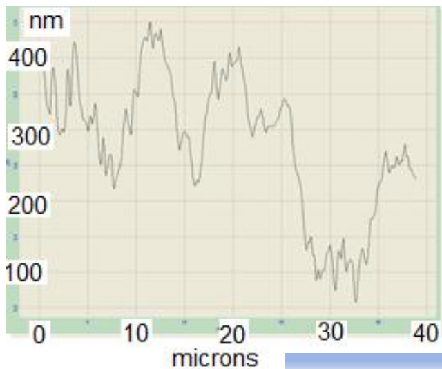
Force microscopy of original FR4
