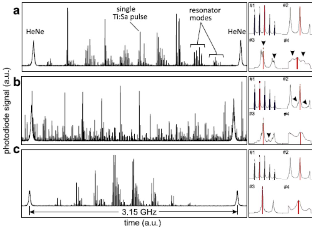
Spectra of the narrow-band Ti:Sa laser recorded with the scanning Fabry-Perot interferometer
