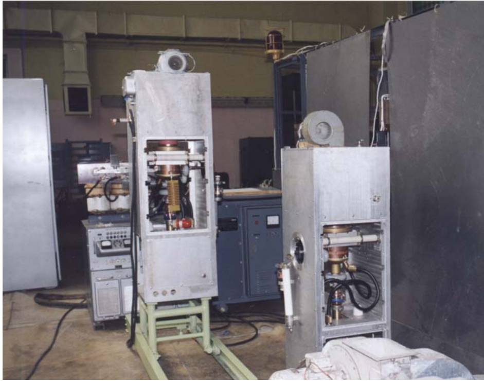
Fig. 5. The external view of the power amplifier, on the back plane is shown the pre-amplifier with the feeder
