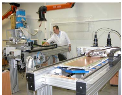
Fig. 7. Automated wire soldering and wire pitch and tension measuring machines at PNPI-1
