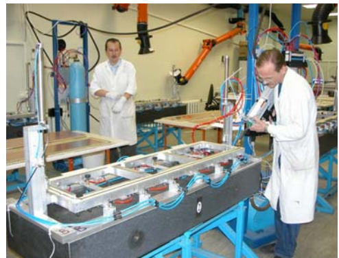
Fig. 6. Bar gluing tables at PNPI-1 facility
