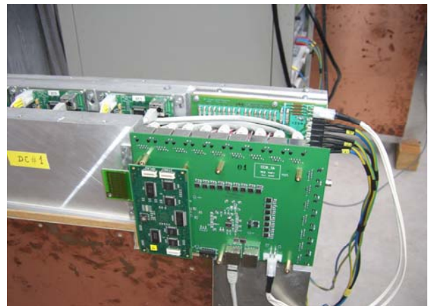
Fig. 2. CROS-3 Digitizers and Concentrator are on-chamber mounted system components
