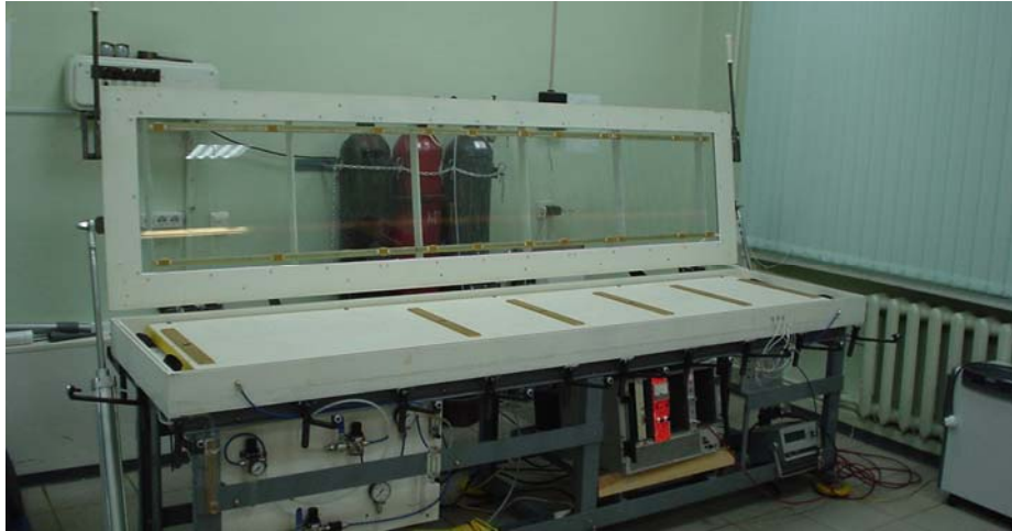
Fig. 4. A view of the high voltage test bed
