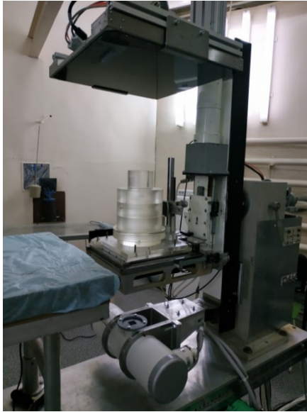
Fig. 5. X-ray centralizer in vertical position
