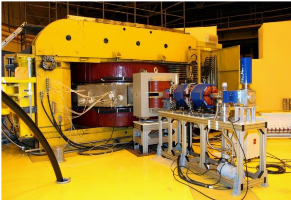
Fig. 1. The external view of the C-80 cyclotron and the beginning line of the transport line
