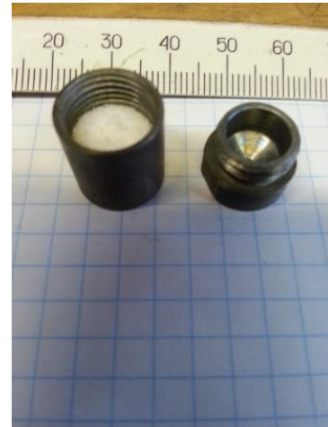
Fig. 2. On the left – the spectrum of the vessel with the irradiated RbCl before heating is shown by squares; the spectrum after one hour vessel heating at a temperature 500 °C is shown by circles. On the right – the vessel with the irradiated RbCl powder after one hour vessel heating at a temperature 500 °C is shown [5]. The RbCl white powder is seen in the vessel
