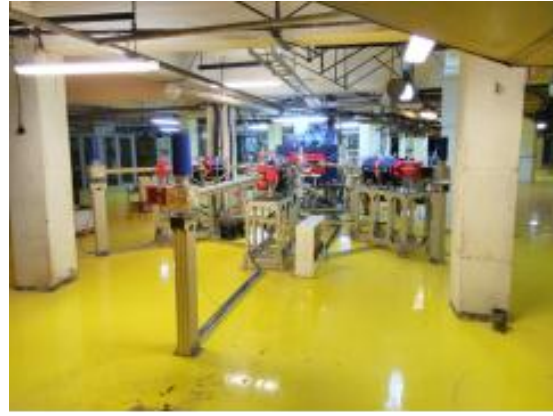
Fig. 1. Cyclotron C-80 (ground floor) with three proton beam lines to the target stations (in the cellar)
