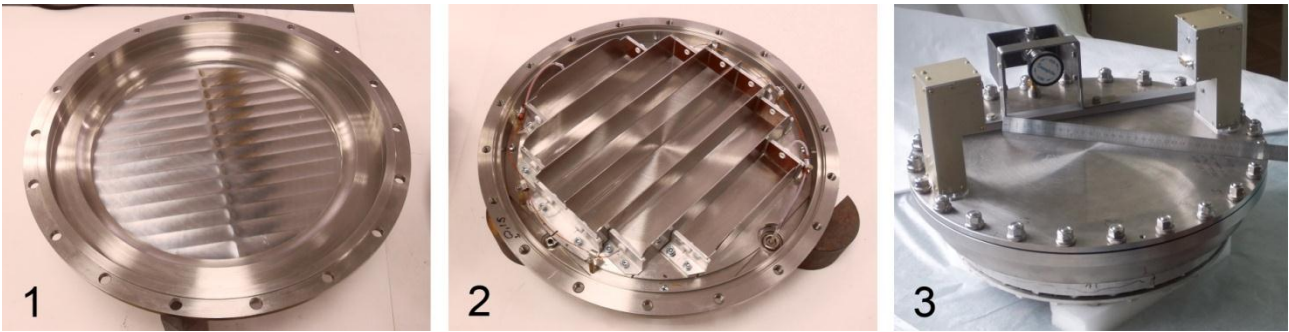
Fig. 1. UCN detector parts: 1 – the upper part of the detector with the entrance window (the grid supporting the entrance foil is seen); 2 – the bottom part of the detector with six proportional counters; 3 – assembled UCN detector, shown from its back side (two preamplifiers and a gas manometer are seen)
