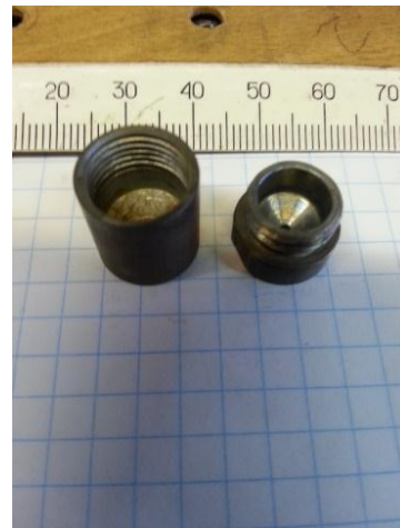
Fig. 3. On the left – the spectrum of the vessel with the irradiated RbCl after its heating at a temperature 500 °C (red dots) and the spectrum after one hour vessel heating at a temperature 900 °C (green dots). On the right – the vessel after one hour heating at a temperature 900 °C [5]. It is seen that practically all RbCl powder was evaporate
