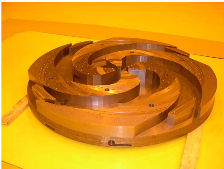
Fig. 6. View of the pole tip for the cyclotron C-80
