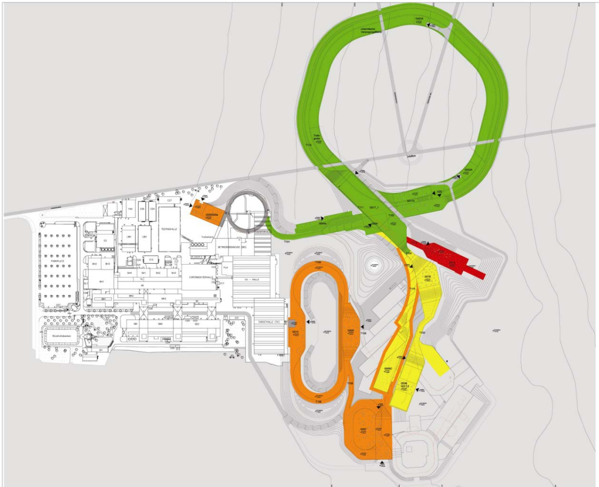
Fig. 1. FAIR MSV. Colouring of modules: 0 – green; 1 – red; 2 – yellow; 3 – orange. Modules 4 and 5 are not marked in colour. Not shown is the additional experimental area above ground, which is a part of Module 1. On the left hand side of the figure, the existing GSI facility is shown
