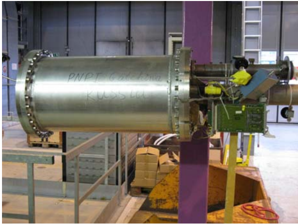
Fig. 7. Prototype of the chamber Actar2 to be placed inside the gamma-spectrometer CALIFA
