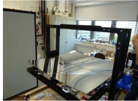
Fig. 14. Real assembly of the four-mirrors mount for the prototype
