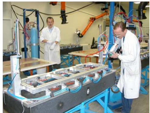
Fig. 6. Bar gluing tables at PNPI-1 facility
