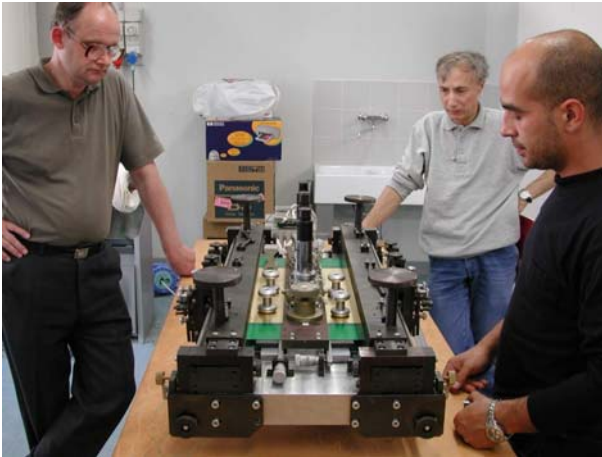
Fig. 2. The PCB trimmers developed for preparation of the slats for stations 3, 4, 5 (left) and for station 2 (right) at PNPI
